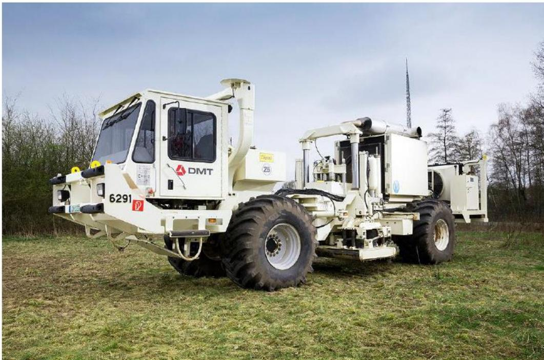
The AHV-IV, coupled with SSC Force 3 GPS Synchronized Source Control Systems, designed for high-productivity acquisition (HPVS), for autonomous acquisition methods and wired and wireless recording operations. Delivers high-quality seismic data to our customers.
